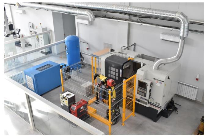
The robotic system combines additive and subtractive technologies, providing process optimization capabilities for multi-purpose tasks. The production of parts via a chip removal process is an economical and widespread technology. It also offers a wide selection of machinable processable materials, tools and processing modes. The combinations of all these possibilities create a huge field for optimization according to various criteria, such as processing time, tool life, etc.
