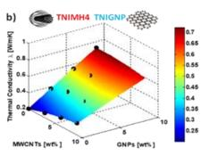
Hybrid nanocomposites of poly(lactic) acid, reinforced with carbon nanotubes and graphene nanoplates, are being developed at the Thermal Conductivity Testing Laboratory using the Light Flash (LFA) technique to determine a set of thermophysical characteristics. A fourfold increase in the thermal conductivity of the nanocomposites was achieved with 9 wt.% graphene nanoplates (GNP) compared to that of unfilled
