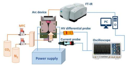
The Laboratory of Plasma Technologies on the Lozenets Campus has established a system for studying the dissociation of  $CO_2$  in a stabilized DC arc discharge at atmospheric pressure. The experimental setup includes the gas supply system, the power supply, the discharge and diagnostic systems - electric current and voltage probes and a Fourier spectrometer to measure the degree of dissociation.
