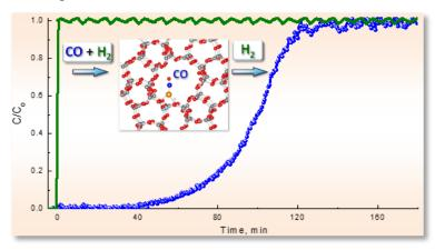
The figure shows the change in gas concentration after passing a gas flow containing hydrogen and carbon monoxide through the Cu/ZSM-5 adsorbent. The hydrogen passes unimpeded while the CO is retained by the adsorbent for about 40 minutes until it is saturated.
