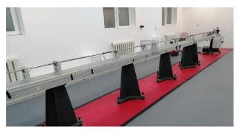
This laboratory possesses a Hopkinson bar system, which is used to obtain the diagram of elastic and plastic deformation under pressure obtained as a result of impact on the specimen with selected parameters. Modulus of elasticity and tensile strength are determined from the diagram. The maximum stress and maximum deformation depend on the selected impact conditions (mass and speed of the striker).
