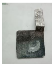
Figure 1: Zn anode (Zn powder + AGAR binder) initial (a) and after 450 cycles (b).
