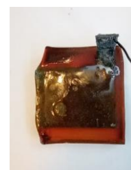
Figure 2: Zn anode (electroplated Zn on Cu foam) initial (a) and after cycling 500 cycles (b).
